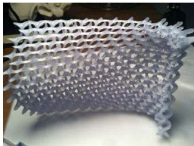
3D printed parametric curtain wall made with Grasshopper Source: http://www.thingiverse.com/thing:119598
