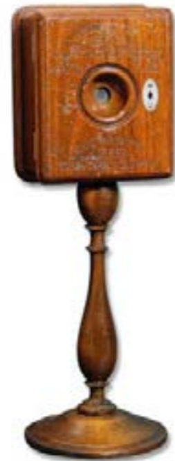
The Blake Transmitter: Invented by Francis Blake as the first successful telephone transmitter Source: http://www.sparkmuseum.com
