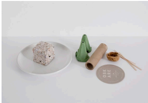
Fig.60: Mycelium inoculated reclaimed paper cube, egg carton pieces, cardboard tube, walnut shell, wooden coffee sticks, beer coaster Photo: Miriam Josi, 2021
