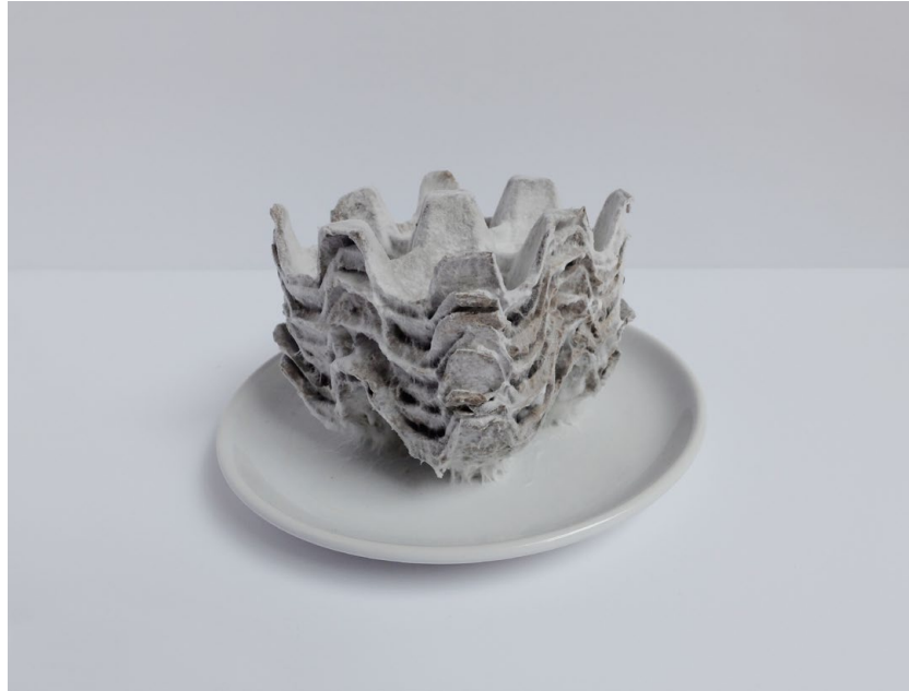
Fig.52: Experiments of mycelium feeding and growing on piled egg cartons assembling them together. Photo: Miriam Josi, 2021
