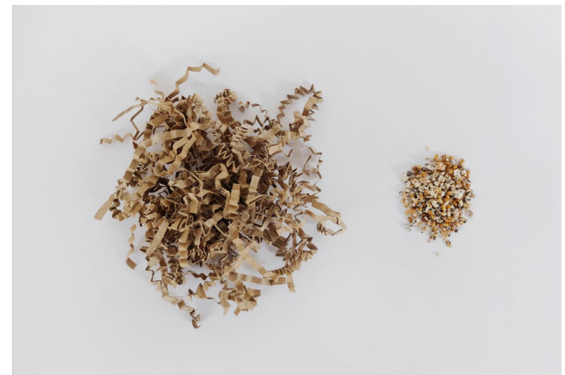
Fig.31: Shredded kraft paper (left) to be mixed and inoculated by pleurotus mycelium spawn (right). Photo: Miriam Josi, 2021
