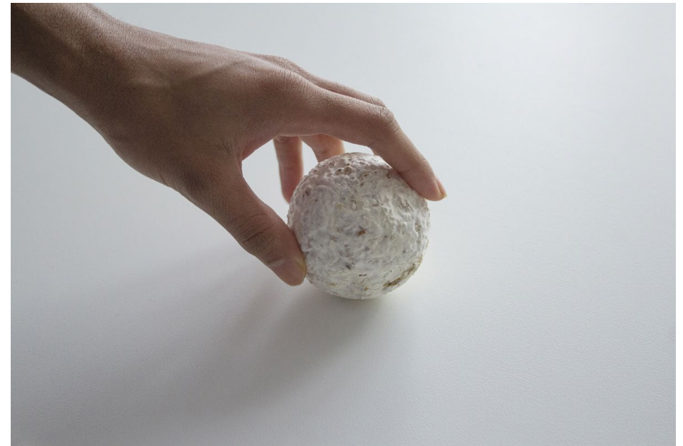
Fig.22: Material sample of mycelium grown on crushed eggshells from an experimental material workshop at Ecole Condé Paris. Photo: Tyrone Fazeuilh, 2020
